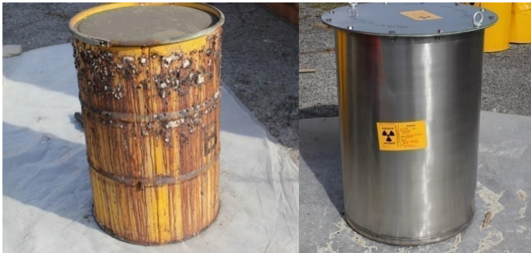
Figure 8 Degraded drums (left), after overpacking with steel drums (right)
